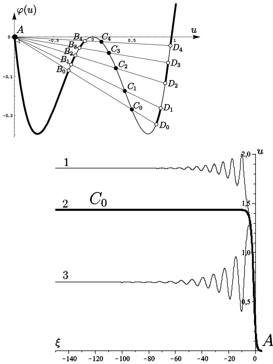
In the figure the structure and phase diagram of the special discontinuity  $C_0$  (bold line) and admissible non-singular discontinuities corresponding to points close to  $B_0$  and  $D_0$  are shown.
