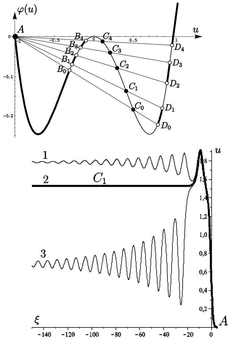
In the figure the structure and phase diagram of the singular discontinuity  $\mathbf{C}_1$  (bold line) and admissible non-special discontinuities corresponding to points close to  $\mathbf{B}_1$  and  $\mathbf{D}_1$  are shown.
