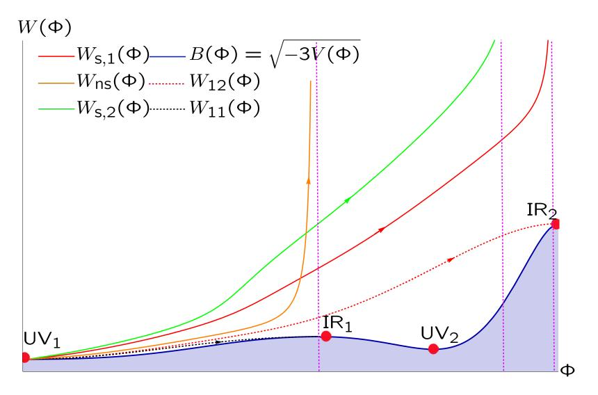
The solid lines represent the superpotential  $W(\Phi)$  corresponding to the three different solutions starting from  $UV_1$  which exist at small positive curvature. Two of them (red and green curves) are skipping flows and the third one (orange curve) is non-skipping. For comparison, we also show the flat RG flows (dashed curves)
