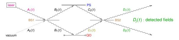
• Interaction light/oscillator:  $C_1(t) = U(t)^{\dagger}B_1(t)U(t)$ ,  $\mathrm{d}U(t) = \cdots$  (Hudson-Parthasarathy equation). Peculiar property:  $U(T)^{\dagger}B_1(t)U(T) = U(t)^{\dagger}B_1(t)U(t)$ ,  $\forall 0 \leq t \leq T$
