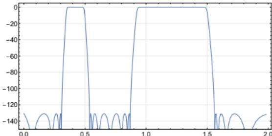
Optimal magnitude response of order 34 with ripple magnitude at the passbands  $-5 \cdot 10^{-5} dB$  and attenuation of  $-130 dB$  at the stopbands
