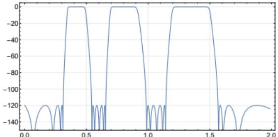
Optimal magnitude response of order 38 with ripple magnitude at the passbands  $-10 \cdot 10^{-5} dB$  and attenuation of  $-120 dB$  at the stopbands
