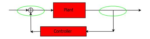
Measurement Based Feedback Control
