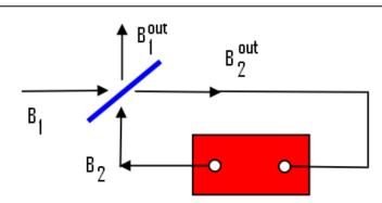
$$dB_2 = S_0 dB_2^{\text{out}} + L_0 dt = S_0 (S_{21} dB_1 + S_{22} dB_2) + L_0 dt$$
