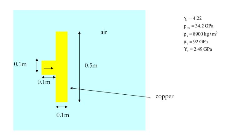
A copper projectile impacts a copper plate at 800m/s
