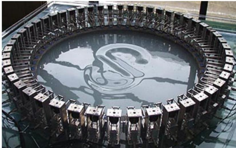
Device uses waves to “print” on water surface
