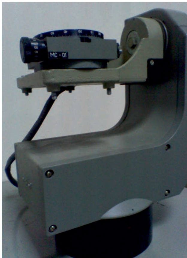
Fig. 13. Simplified Stage for MAGMCC_CCI – Multi-Axis Goniometric Microscopy in Cylindrical Coordinates for Chromatographic Column Imaging
