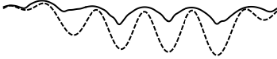
Fig. 8. (Dashed curve) cross section of 3D image of initial surface relief obtained at the cooperative nucleation stage; (full curve) surface relief obtained by computer simulation of the KPZ equation (14) with \delta = 10^{-2} at T_{growth} = 85
